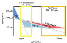
Fig.1 Capacity (mA/h) vs Output (mA)
