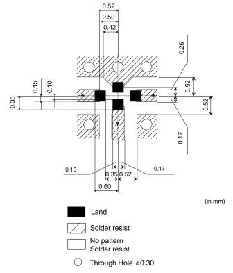
$<sup>^{\</sup>star}$  Line width to be designed to match  $50\Omega$  characteristic impedance, depending on PCB material and thickness.
