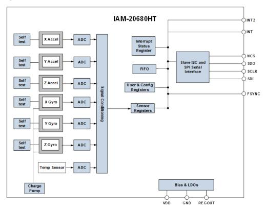
Figure 5. IAM-20680HT Block Diagram
