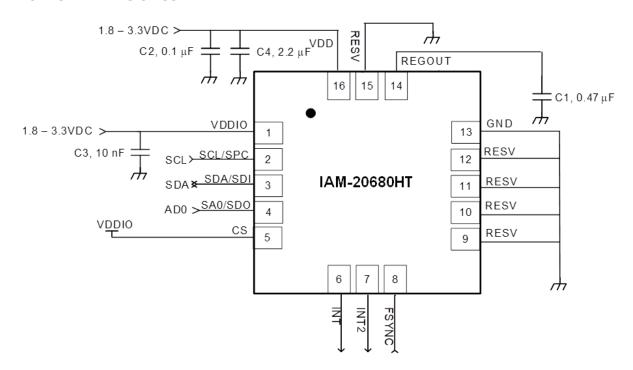
Figure 4. IAM-20680HT LGA Application Schematic
