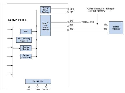
Figure 6. IAM-20680HT Solution Using I<sup>2</sup>C Interface
