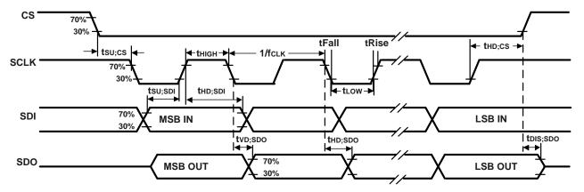
Figure 2. SPI Bus Timing Diagram
