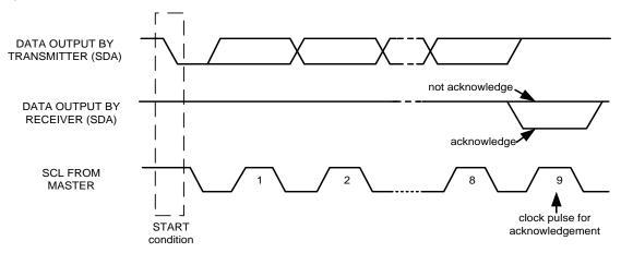
Figure 9. Acknowledge on the I<sup>2</sup>C Bus
