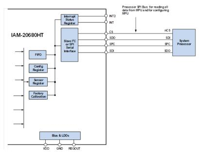
Figure 7. IAM-20680HT Solution Using SPI Interface
