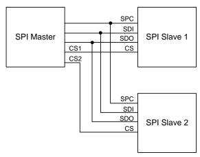
Figure 11. Typical SPI Master/Slave Configuration
