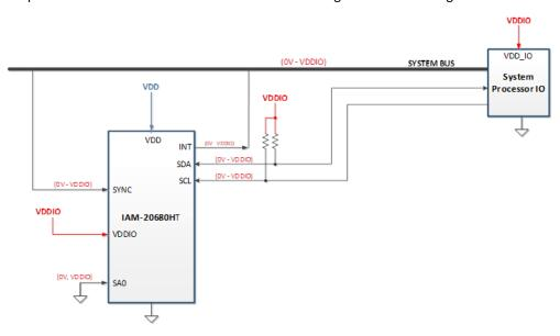
Figure 12. I/O Levels and Connections
