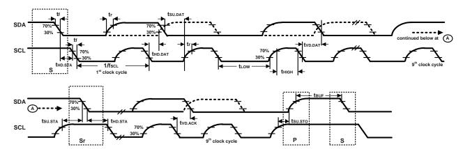
Figure 1. I<sup>2</sup>C Bus Timing Diagram
