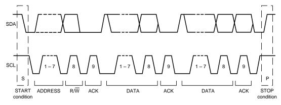
Figure 10. Complete I<sup>2</sup>C Data Transfer
