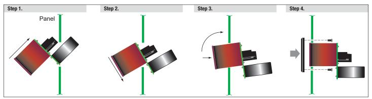
Figure 2. Panel Installation
